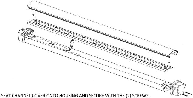
INSERT DIFFUSER INTO THE GROOVE IN SECURED ENDCAP.
